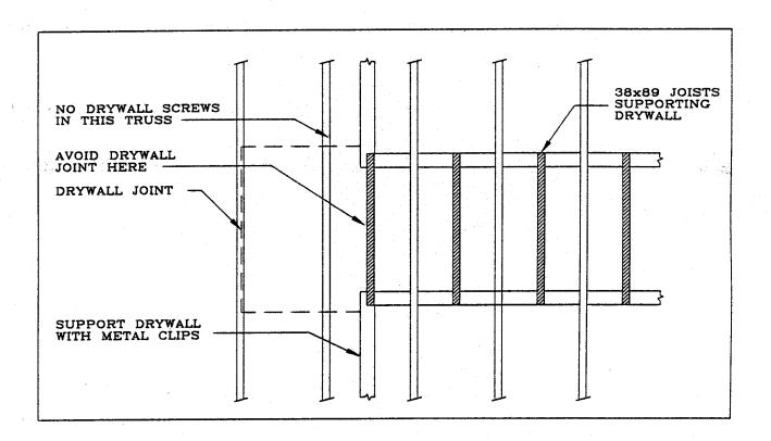
Special cases occur where ceilings are partially vaulted. The following illustrations indicate potential solutions involving partitions that are framed through to the underside of the sloping portion of the bottom chords of the trusses.
