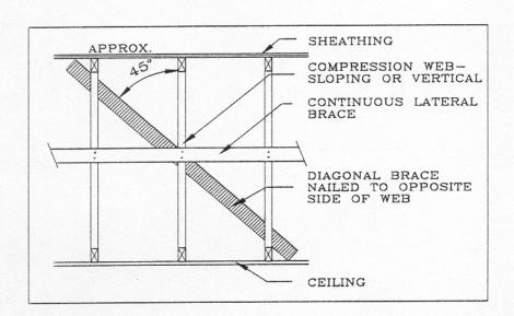
The frequency at which the diagonal or tie-back braces should be installed is governed by the ability of the nails in the diagonal brace to transfer the loads. Assuming the use of two nails at each connection, the necessary frequency of the diagonal braces can be determined by the following formula:
