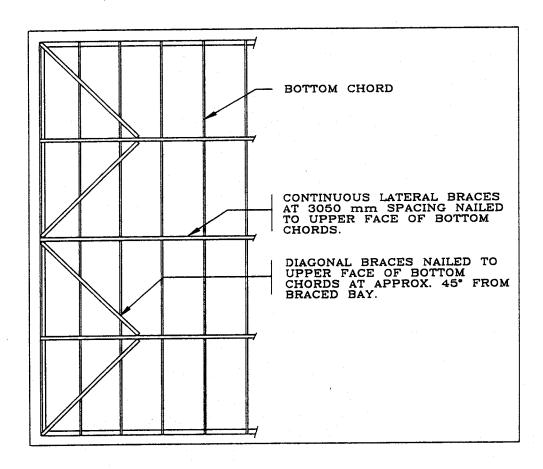
For multiple bearing trusses or cantilever conditions, portions of the bottom chord become compression members and should be laterally braced to resist buckling in the same manner as the top chords. Truss design drawings show the maximum spacing of lateral braces in these cases, assuming no rigid ceiling material will be installed.
