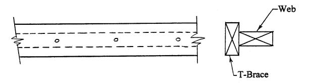
Nailing - 3" common wire nails at 6" o.c. or 3 1/4" - 0.12" diam. power driven nails at 4" o.c.
